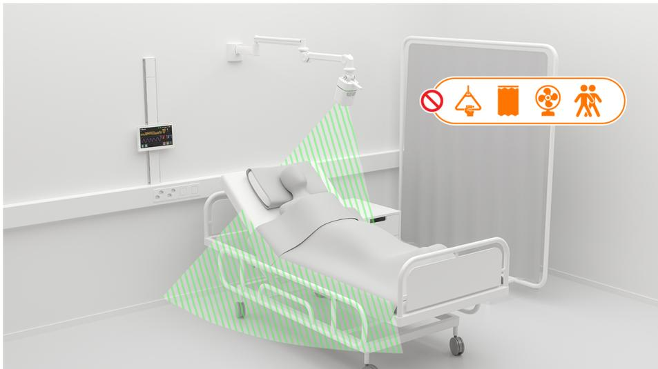
The sensor unit should be positioned so that patient's chest stays within the optimal zone even if they move around in bed, sit up or lie down. This ensures the highest accuracy in readings.
