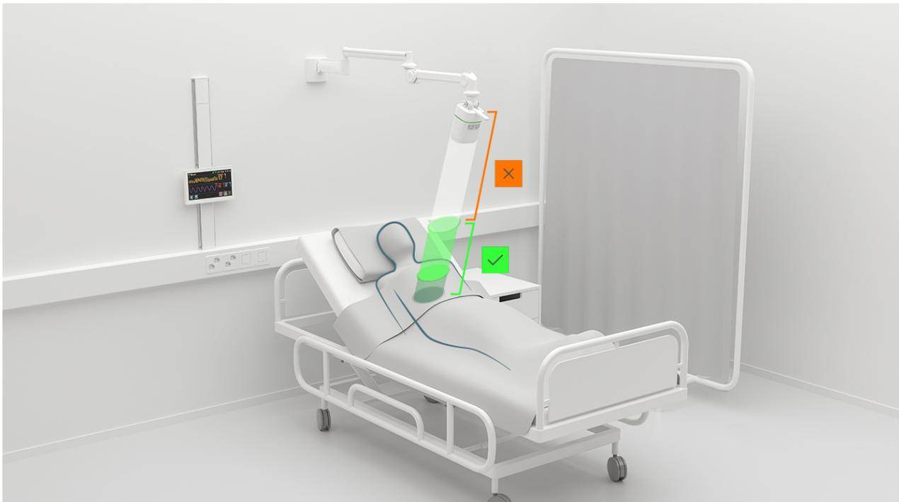
Keep in mind that the monitoring distances may affect the ways in which the sensor unit can be positioned in any given environment. Do not set a distance that cannot be adhered to, for example: the maximum distance must not be so long that it continuously registers nearby patients, objects or people. For details on the monitoring zones affected by the maximum monitoring distance and what you should take into account, see "Instructions for Use", section "Monitoring zones".
