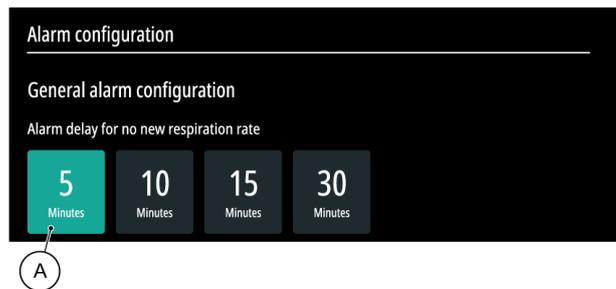
If the system, over a period of time, does not obtain new respiration rate measurements, a technical alarm becomes active. The time duration before generating the alarm for no new respiration rate is configurable, and by default set to five minutes.
