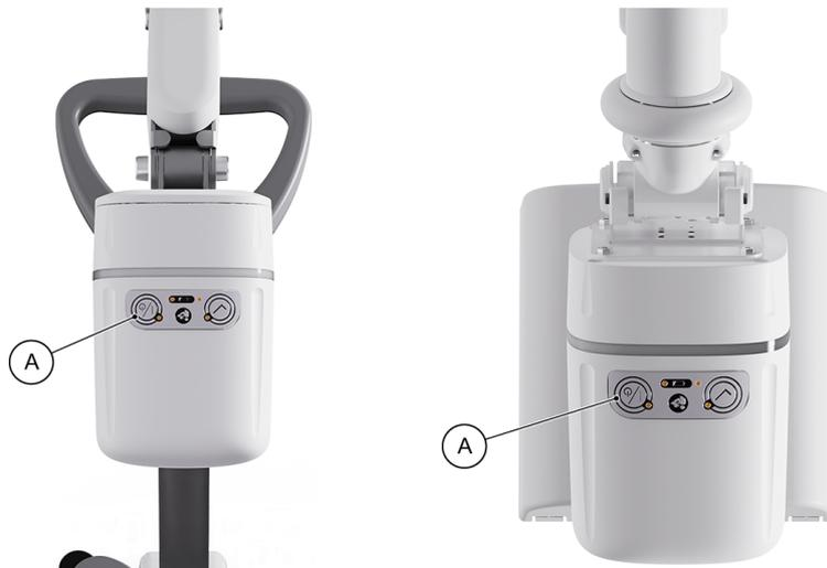
No specific actions are required to initiate the system self-test. Turn the sensor unit off by keeping the on/off button (A) pressed, and then on again with the same button, and the self-test runs automatically.
