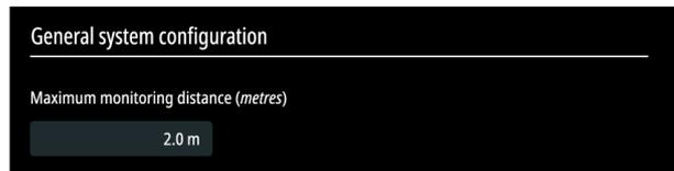
Set the preferred maximum distance between the sensor unit and the patient. The distance should be set so that the patient's chest area is always within this distance as measured from the back of the sensor, even if they move in the bed, lie down or sit up.
